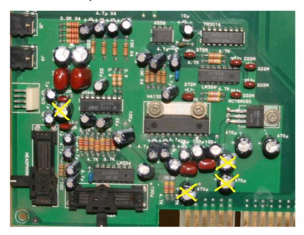
The capacitors that do not get replaced are used for filtering the +5v and +12v power lines.
