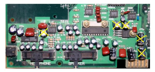
The capacitors that do not get replaced are used for filtering the +5v and +12v power lines.
