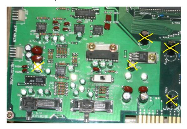
The capacitors that do not get replaced are used for filtering the +5v and +12v power lines.
