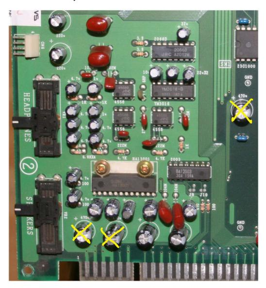
The capacitors that do not get replaced are used for filtering the +5v and +12v power lines.
