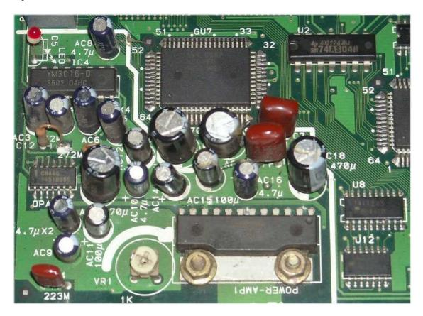
Every cap that is soldered to the heavy ground plane on the top of the board will require extra amounts of heat to desolder. You may find it easier to heat up the ground leg of the capacitor with a soldering iron then pulling it out and desoldering the hole afterwards.
