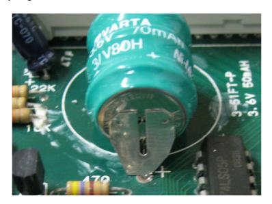
At this point the battery can be soldered in place on the 4 slot boards. After this there is still something else to do. The battery sits too tall on the board and will interfere with the fit of the top board. The legs will need to be bent on the battery to snug it to the bottom board and give the clearance needed for the top board to properly fit.
