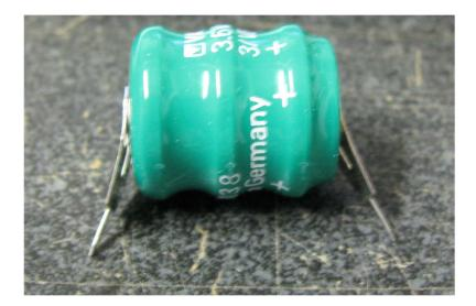
Test fit the battery and look for any possible short circuits. The 4 slot board has traces that run close to the positive terminal on the battery. The lead from the battery could cut through the protective coating on the traces and short circuit them which would result in a board failure.
