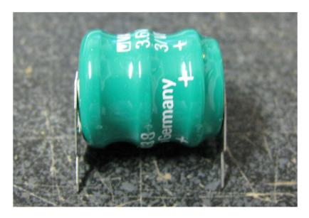
The holes in the board are wider than the battery, but it will fit fine. Simply bend the leads out slightly to line them up with the holes on the game board.
