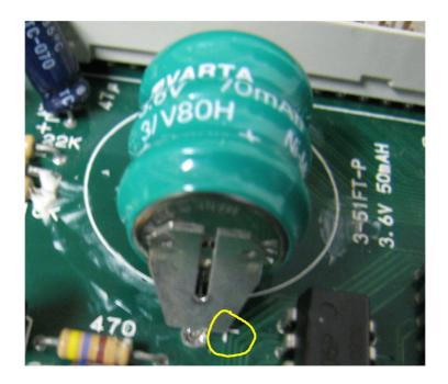
If there is no interference between the battery and the traces then solder the battery in and reassemble the system. Don't forget to reset the Backup RAM and set the clock. You are done UNLESS it's a 4 slot board! These will need further modification.
