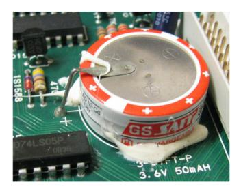
Next remove the red cardboard protecting the battery leads on the bottom from shorting out. You can either remove the whole piece or if you are careful enough, cut out a small section to expose the solder joints for the battery. Removing a small section is preferred as it can be easily put back in place with a bit of electrical tape covering it but you run a high risk of cutting circuit board traces under the cardboard.
