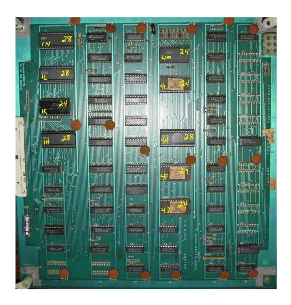
Next, replace the SIP resistor packs on the video board. There are only 8 to replace on the Video board.
