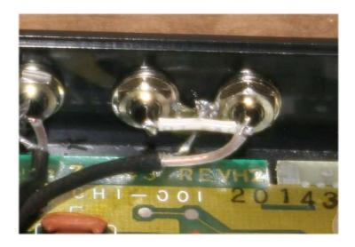
Trim back about 1/4" of insulation from the other end of the LONG piece of thin coaxial cable. Use a needle or pointed PCB tool to separate the ground braid away from the center conductor. Tin the wires and the pins on the chip to make this step easier.
