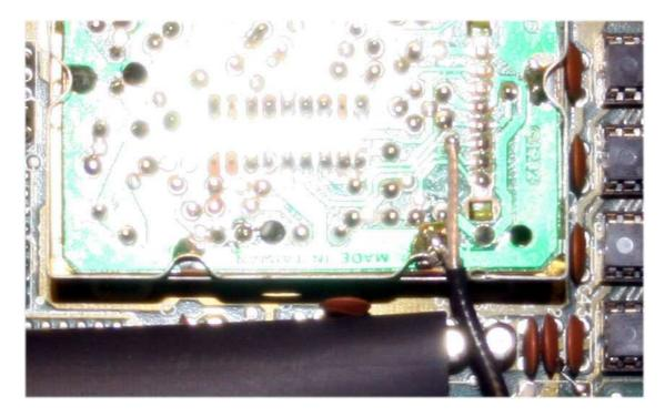
Put the cover back on the RF modulator. If it doesn't fit, ensure the sides of the modulator where it was cut for the coaxial cable are straight.
