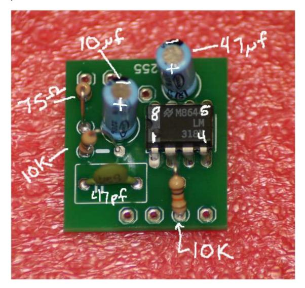
The resistors are color coded for identification. Full resistor color code charts are available on the internet.
