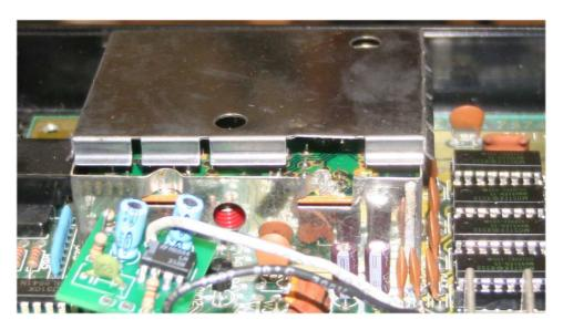
Trim back about 1" of insulation from the other end of the thin coax that is connected to the inputs on the video mod board. Separate the braid from the center conductor.
