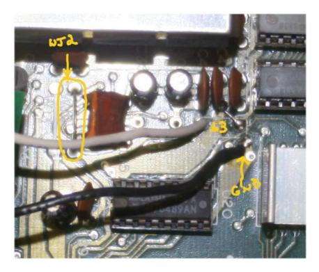
Solder the +12v and the ground wires to the video mod board. The wires should lay so they go to the right of the board. This will make it easy to install the heat shrink tubing over the mod board when finished.
